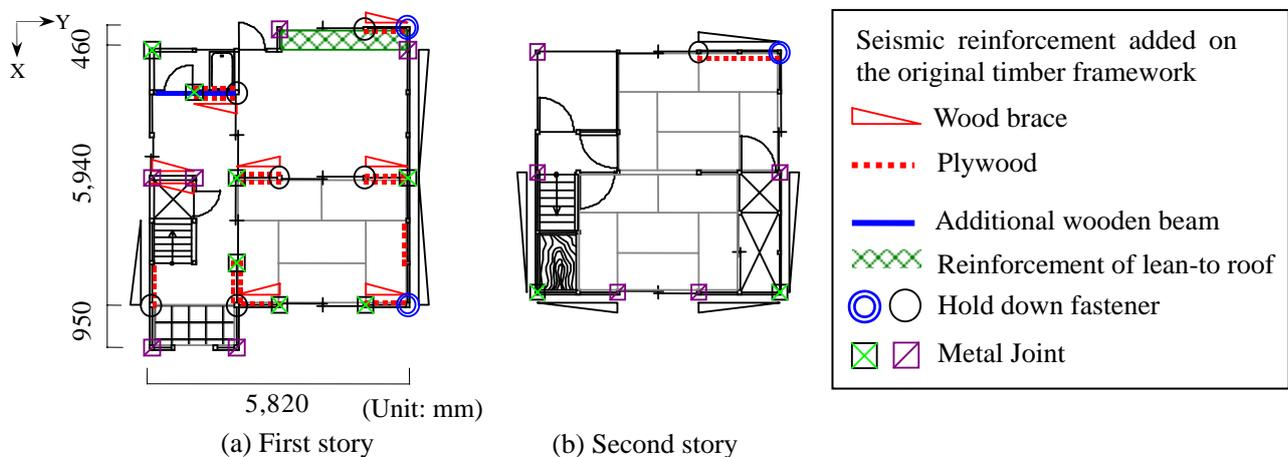
Fig.2 Plan of Model B
