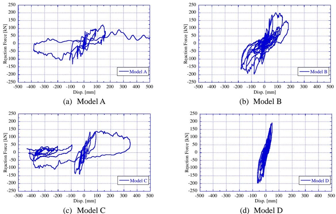
Fig. 4 Load-displacement relationship of each model after the first 100% JR Takatori excitation
