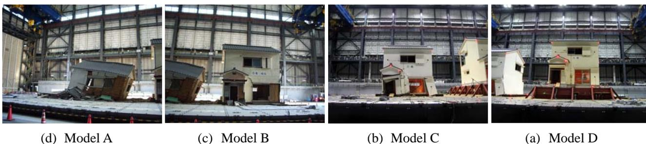
Fig. 3 Damage of each model after the first 100% JR Takatori excitation
